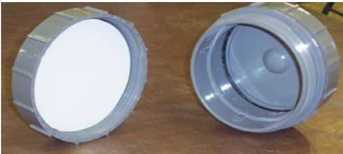
Circular gelcoat panels used for 12 month blistering test in de-ionised water.
